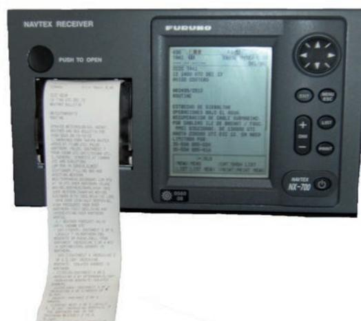
Figura 2. Foto receptor NAVTEX
